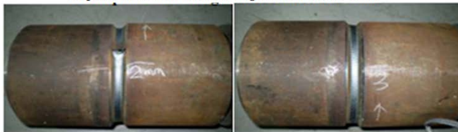
Root pass welding – front side
