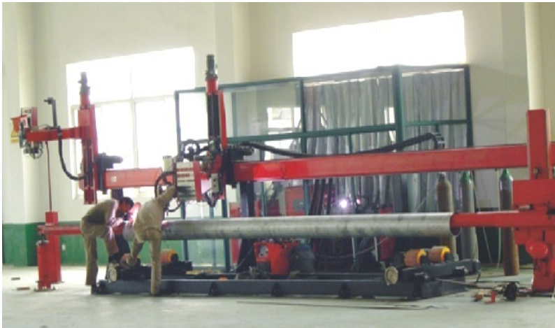
Longitudinal seam welding system
