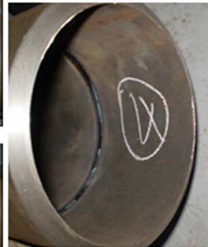
Root pass welding – back side
